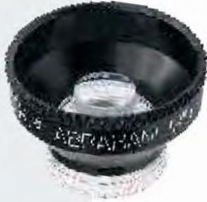
A 66D magnifying lens for viewing the patient's iris. The power density of the laser beam at the iris is increased 2.5x compared with a flat lens. A 50 micron spot size setting yields a 31 micron spot on the iris. The lens provides additional safety by reducing the power density at the cornea and retina by 2.8x.
